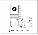
**3** Hold down the light/programming button again for 3 seconds. A short acknowledgement tone is audible. At the bus telephones, a different tone sequence is audible when a call is placed by this door station.
