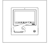
**3** Tap Settings; > Installation; > Start Programming; > Start. The bus video panel establishes the speech connection to the door station. The bus video panel is now in the programming mode.
