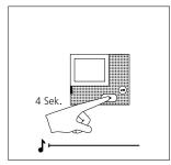
Hold down the speech button for 4 seconds. A protracted acknowledgement tone sounds as confirmation and the muting LED begins to flash. The bus indoor device establishes the speech connection to the door station. The bus indoor device is now in the programming mode.
