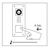
On the door station, press and hold the desired call button for 4 seconds until a sustained tone can be heard from the door loudspeaker. The call button is now assigned to the bus indoor device.
