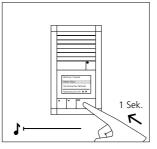
5 When the selected name is shown on the display, press the OK button on the DRM 612-..., a protracted tone can be heard at the door loudspeaker. The selected name is now assigned to the bus indoor device. The speech connection is interrupted. If the name was already programmed, the OK button must be pressed twice.
