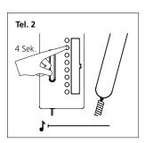
**4** Lift the receiver at the second bus telephone which you wish to program. Hold down the light button for 4 seconds. Do not replace the receiver!
