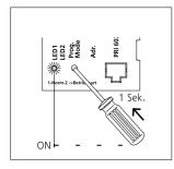
Switch on the programming mode. At the BNG/BVNG 650-..., press the programming mode button briefly. The LED 1 flashes in a 2-second rhythm to indicate that the programming mode is active.
