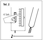
**8** At the second bus telephone, hold down the internal call button you wish to use to call the first bus telephone for 4 seconds.
