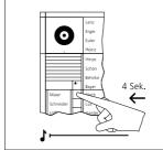
**5** At the door station, hold down the required call button for 4 seconds until a protracted tone sounds at the door loudspeaker.
