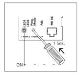
**1** Switch on the programming mode. At the BNG/BVNG 650-..., press the programming mode button briefly. The LED 1 flashes in a 2-second rhythm to indicate that the programming mode is active.
