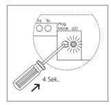
Switch the BSE 650-... to the programming mode. To do this, briefly press the programming mode button with a small screwdriver. The LED flashes slowly.
