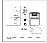
**3** Press the programming button for 4 seconds. The In-Home LED then flashes in a one-second rhythm. The Smart Gateway is now in the programming mode.
