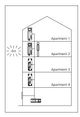
**3** Set up the bus telephone in apartment 2 with the receiver in place, the storey call sounds as an acknowledgement tone and the LED of the muting button flashes.
