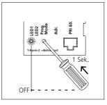
**5** The call button is now firmly assigned to the Smart Gateway/ Smart Gateway Professional.
