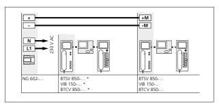
A maximum of 1 VIB 150-.../BTSV/BTCV 850-... unit can be supplied by a NG 602-... line rectifier. If several bus telephones have to be simultaneously rung using one bell button, each VIB 150-.../BTSV/BTCV 850-... must have its own NG 602-...
