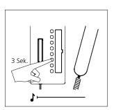
**4** Pick up the receiver on the bus telephone and press the button for which the control function is to be deleted for 3 seconds.
