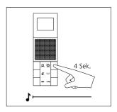
6 Video indoor station 2: Hold down the internal call button you wish to use to call the first device for 4 seconds. A protracted tone is audible. The buttons are now programmed at both devices.
