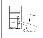
**3** Hold down the call button you wish to assign to one or more in-house telephones for 3 seconds. (e.g. door call 1 to telephone 1).
