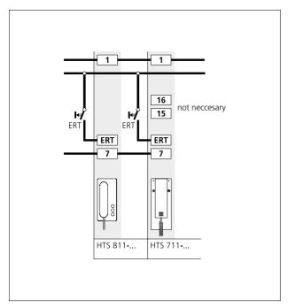
The in-house telephones HTS/HTC 811-... can be used in existing 1+n systems with the predecessor models HTS/HTC 711-... Exchange of HTS/HTC 711-... units for HTS/HTC 811-... units is possible. The terminal designations of the in-house telephones are identical. The HTC 811-... deviates from the HTC 711-... in as far as the light button can optionally be used as button 1. Switchover takes place via a DIL switch in the in-house telephone HTC 811-...
