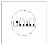
2 Select the relevant telephone using the DIL switch e.g. telephone 1 (DIL 1 ON). Several DIL switches can be used.
