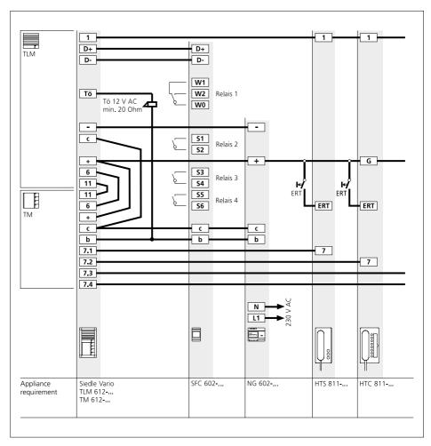
Connection of an SFC 602-... All connected in-house telephones can initiate switching functions of the SFC 602-...
