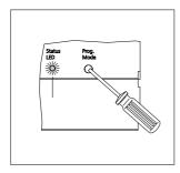
**1** Activate the programming mode at the GC 612-..., the status LED starts to flash.
