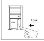
5 The call button you wish to assign to the telephone should be held down for 3 seconds (e.g. door call 2 to telephones 3 and 4). Program other call inputs using the same procedure. Once all the telephones have been assigned, terminate the programming mode.
