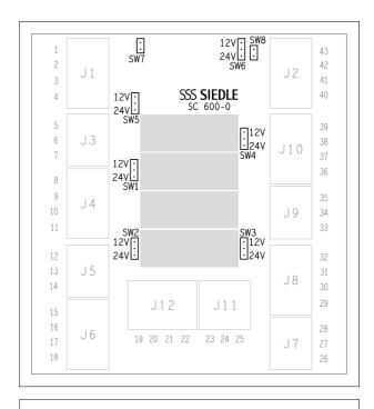
Jumper view – lower circuit board: Processor unit
