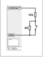
This circuit requires an end of line resistor and an alarm resistor: The alarm resistor and contact are connected in parallel. The end of line resistor is connected in series with the parallel connection.
