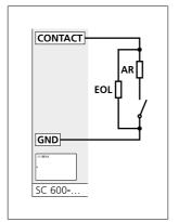
This circuit requires an end of line resistor and an alarm resistor: The alarm resistor and contact are connected in series. The end of line resistor is connected in parallel to the series connection.
