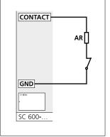
In this circuit, an alarm resistor is located in series with the trigger contact.
