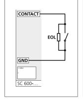
In this circuit, an end of line resistor is located in parallel to the trigger contact.
