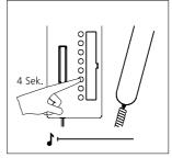
**5** At the bus telephone, hold down the button you wish to use to call the door station for 4 seconds. Replace the receiver. The button is now assigned to the door station. The door loudspeaker can be dialled at any time.
