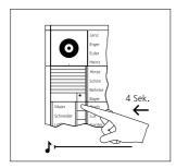
**4** At the door station, hold down the required call button for 4 seconds until a protracted tone sounds at the door loudspeaker.
