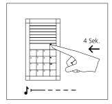
At the door station, hold down the light/programming button for 4 seconds. A protracted acknowledgement tone is then audible which is repeated every 5 seconds as long as the programming mode remains active.
