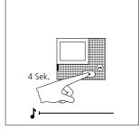
**3** Hold down the speech button for 4 seconds. A protracted acknowledgement tone sounds as confirmation and the muting LED begins to flash. The bus indoor device establishes the speech connection to the door station. The bus indoor device is now in the programming mode.
