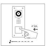
At the door station, hold down the top bell button for 4 seconds. A protracted acknowledgement tone is then audible which is repeated every 5 seconds as long as the programming mode remains active.
