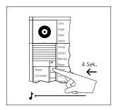
**4** Press the button to which you wish the relay to be assigned and hold down for 4 seconds. A protracted acknowledgement tone is audible in the receiver.
