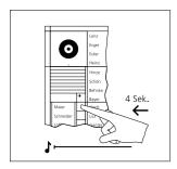
4 On the door station, press and hold the desired call button for 4 seconds until a sustained tone can be heard from the door loudspeaker. The call button is now assigned to the bus indoor device.
