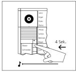
**5** On the door station, press and hold the desired call button for 4 seconds until a sustained tone can be heard from the door loudspeaker. The call button is now assigned to the bus indoor device.
