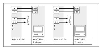
A maximum of 1 BVPC 850-... can be supplied with a PSM 1 12 24 line rectifier. In systems with bus video panel, a maximum of 2 PSM 1 12 24 may be used.
