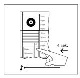
On the door station, press and hold the desired call button for 4 seconds until a sustained tone can be heard from the door loudspeaker. The call button is now assigned to the bus indoor device.
