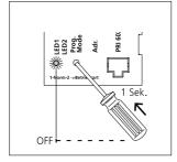
**5** The call button is now firmly assigned to the bus indoor devices.
