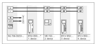
A maximum of 3 VIB 150-.../BTSV/BTCV/BVPC 850-... units can be supplied by a NG 706-30/33-... line rectifier. The specified ranges only apply to the external power supply to the devices, not to the ranges of the In-Home bus. Ranges applicable for J-Y(St)Y or YR installation cable with 0.8 mm core diameter! Only bus indoor devices which are located in the same line can be supplied by one line rectifier.
