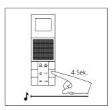
2 Video indoor station 1: Hold down the light button for 4 seconds. A protracted acknowledgement tone sounds as confirmation and the muting button begins to flash.
