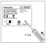
2 At the BVM 650-... hold the programming button down for 4 seconds. After this, the status LED flashes at short intervals as long as the programming mode is active.
