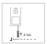
**2** At the door station, hold down the programming button for 4 seconds. A protracted acknowledgement tone is then audible which is repeated every 5 seconds as long as the programming mode remains active.
