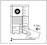
**5** On the door station, press and hold the desired call button for 4 seconds until a sustained tone can be heard from the door loudspeaker. The call button is now assigned to the bus indoor device.
