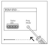
**3** Activate delete mode, to do so press the programming mode button on the BSM 650-... with the screwdriver until all four LEDs light up for 3 seconds and then flash.
