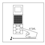
**3 Video indoor station 1:**Hold down the light button for 4 seconds. A protracted acknowledgement tone sounds as confirmation and the muting button begins to flash. The video indoor station establishes the speech connection to the door station. The video indoor station is now in the programming mode.
