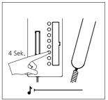
**5** At the bus telephone, hold down the button you wish to use to call the external camera for 4 seconds. Replace the receiver at the bus telephone. The button is now assigned to the external camera. The external camera can be selected at any time.
