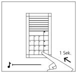
5 Once the required call number has been entered, hold down the button with the bell symbol on the COM 611-..., a protracted tone can be heard at the door loudspeaker. The selected call number is now assigned to the bus indoor device. The speech connection is interrupted.
