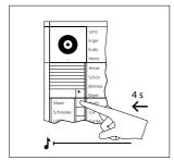
**4** On the door station, press and hold the desired call button for 4 seconds until a sustained tone can be heard from the door loudspeaker. The call button is now assigned to the bus indoor device.
