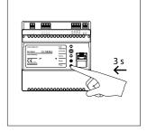
**3** The In-Home LED at the Gateway lights up in green (ready for operation). Press the Prog. button at the Gateway for 3 seconds. The In-Home LED then flashes green.
